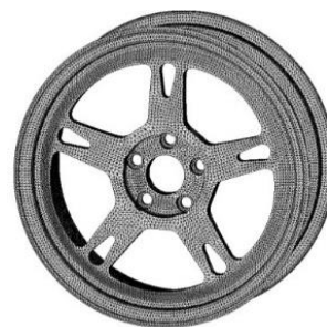
Figure 23: Re-meshed model of wheel
